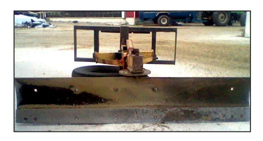
Manita's "feed scraper" was originally a land leveller for the back of the tractor. She made a few modifications, like changing the hook up for the front of the tractor and making it able to swing easily from side to side for good reach on both sides of the aisle.
