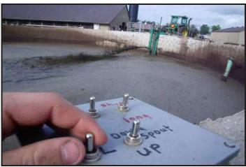
Sand manure is difficult to remove from a manure tank. One method is to use two agitators to keep the sand in suspension. But you have to walk back and forth between the two tractors to control the direction of the pump. My invention allows you to control both pumps from the same location.
